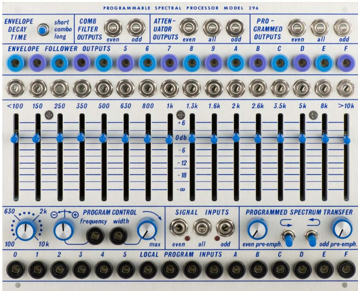
The PROGRAMMABLE SPECTRAL PROCESSOR MODEL 296 is an elaborate set of filters with a number of different outputs and special functions. Perhaps its most obvious function is that of a sixteen band graphic equalizer. The sixteen bands are labeled in hex (0 through F) at the top and bottom of the module and the center frequency of each band is indicated above each slider attenuator.
